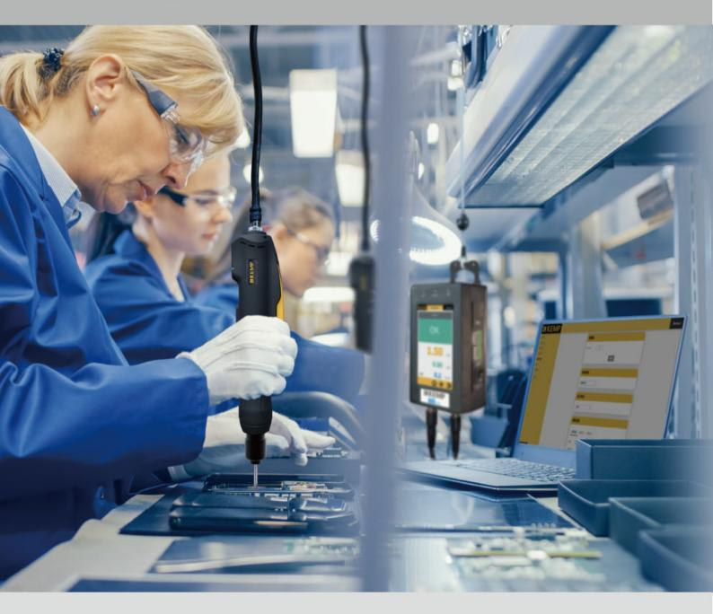
KEMP ideal solution for Industry 4.0 production line. We provide immediate feedback on each tightening process. ETS screwdrivers work in combination with control units together. Their built-in transducer continuously reads torque and position of the screw and sends the gathered data to the controller for analysis.
